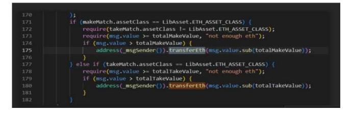
A ".call" is used to transfer coins without gas limit which is being called via library in line no 175 & 180 in ExchangeV2Core.sol.
